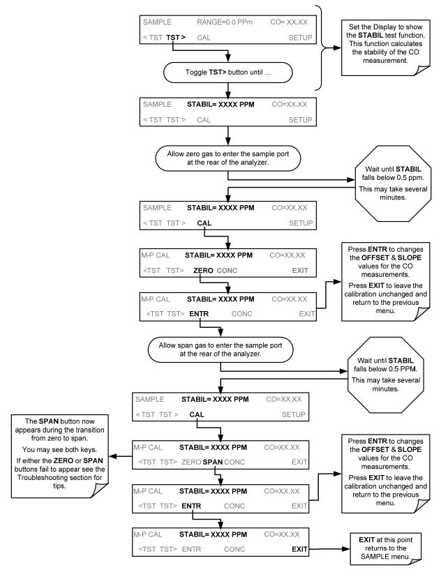
Figure 3-28: Zero/Span Calibration Procedure
